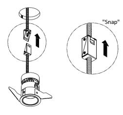
5 WARP CLIPS THEN PUSH LIGHT ENGINE ASSEMBLY INTO CEILING.
